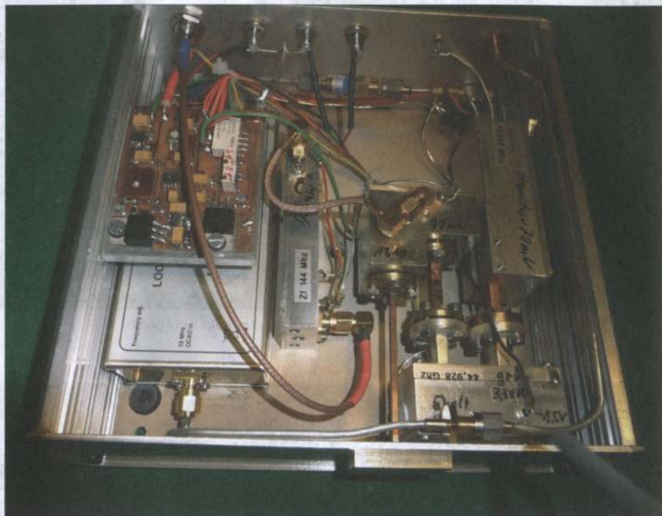
Fig. 6: Completed 134 GHz transverter
