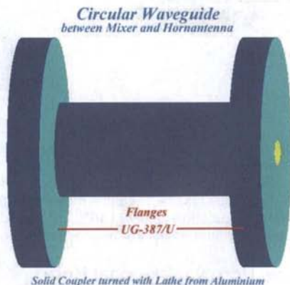
Fig. 8: Possible realisation of the WG adapter in Fig. 7
