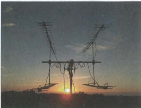
CT1HZE's 4 x 23 el temporary 70cm EME setup in October 2012, beaming west over the Atlantic Ocean
