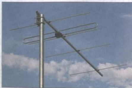
Fig. 1: Foremast mounted 5 ele. version
